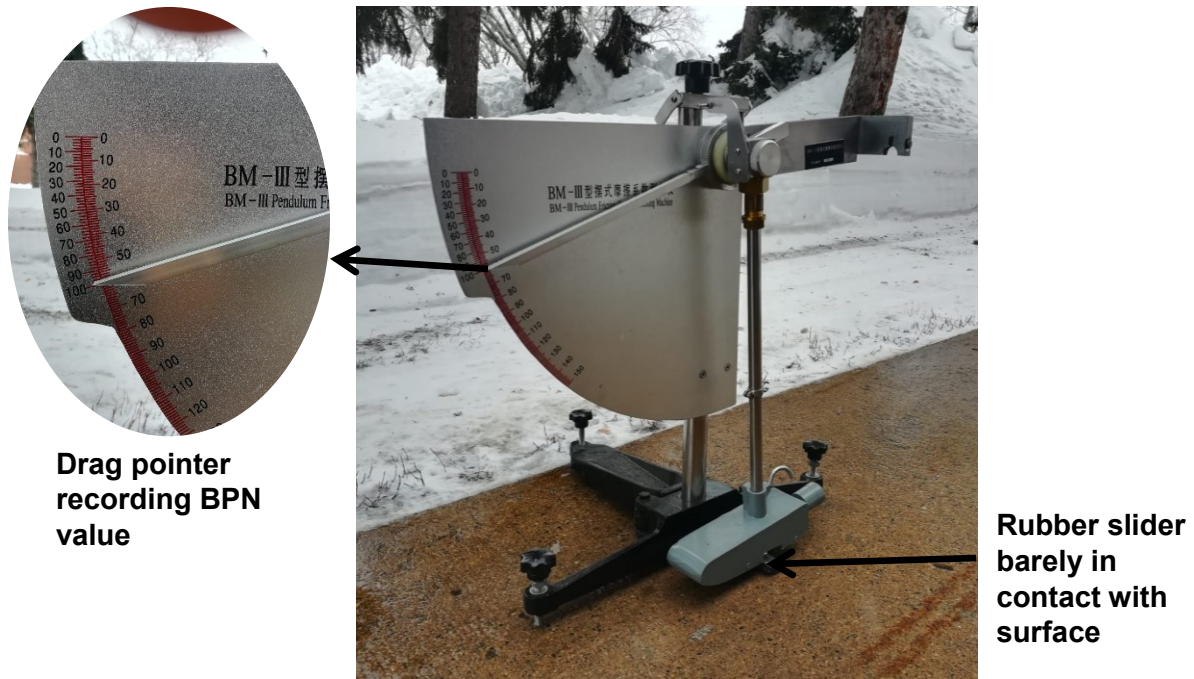
Figure 4.2. British Pendulum Tester for measuring skid resistance of pavement surface.
